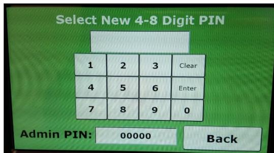
This menu allows the Supervisor to set a unique PIN between 4 and 8 digits long. The current PIN is displayed at the bottom of the screen. If the PIN is lost the Supervisor may contact BenchMark for instructions to access the system.
