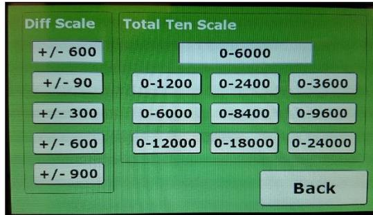
This menu is selected via the Tension menu and is used to set the scales displayed on both Meters.
