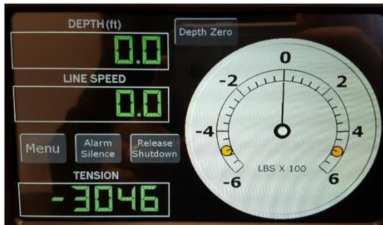
Both Displays are capable of running independently as shown. This allows the operator to continue work in the event of a cracked display or error. This mode allows the operator to see Depth, Tension, Linespeed, and Differential tension all on one screen.
