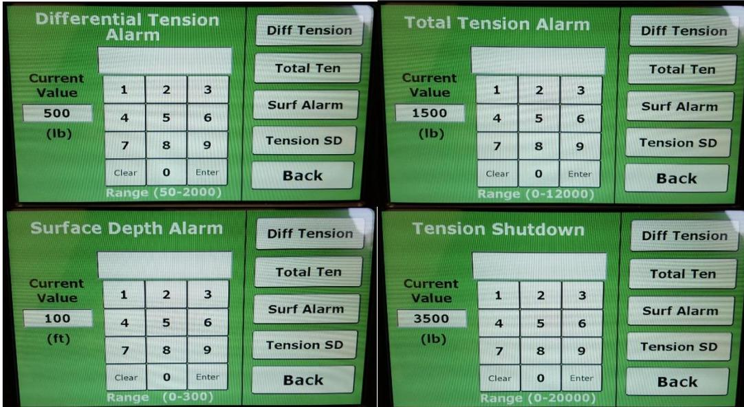
These four menus are selected by pressing the correlating menu button on the right hand side. The operator sets these values and the Dynamic Display alerts are automatically adjusted.
