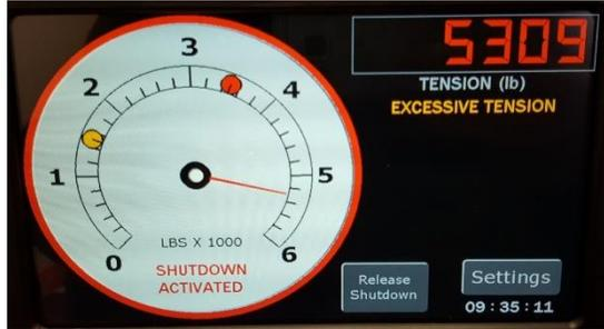
The right screen will also change both the digital display and the bezel to RED if the shutdown condition is met, as well as display a Shutdown message as shown.
